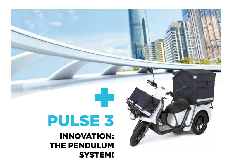
Easy handle, safe and simple to drive, **PULSE 3** is a 3-wheel electric vehicle equipped with a **pendulum system** allowing the driving position to tilt by +/- 30° when turning, which ensures perfect stability when driving or at a standstill. **As the rear part stays stable around bends,**
